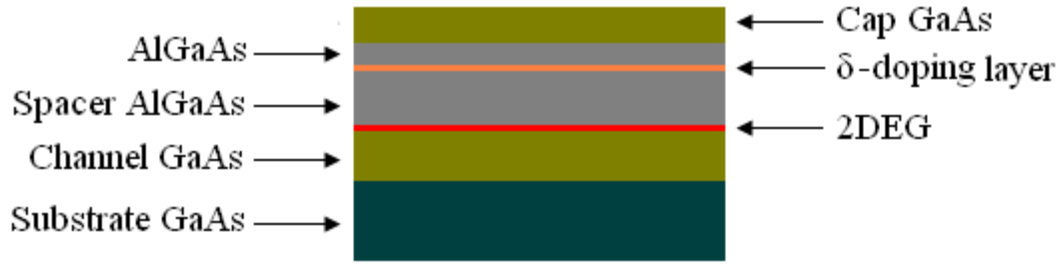
( a ) cross section of GaAs/AlGaAs heterostructure
